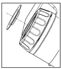
Fig. 13: Aligning the seal
