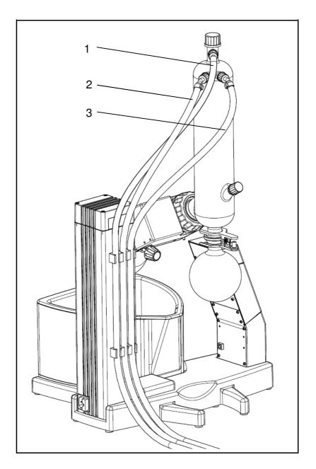
Fig. 5: Attaching lines for coolant and vacuum
